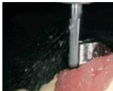
2_ The Friadent telescopic abutments are milled on the model with a turbine and water cooling
