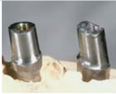
6_ The surface is smoothed with finer cutters and the hollow channel refined. The welding seam cannot be recognized
