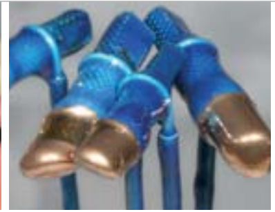
8_ The electroplated secondary parts are shaped to match the set-up
