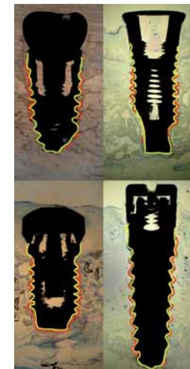
Fig. P9-2: Reduced image of the histological preparation of four different implant types/surfaces labeled to measure the bone-implant contact rate after six weeks. (top left: Branemark, top right: Osseotite, bottom left: XiVE® and bottom right Compress).
